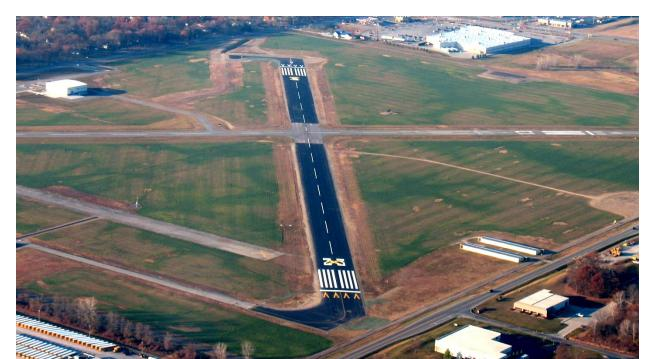
Figure 2-3. Markings for a Temporarily Closed Runway
