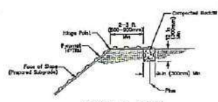
FIGURE 2: INITIAL TRENCH AT TOP OF SLOPE DETAIL
