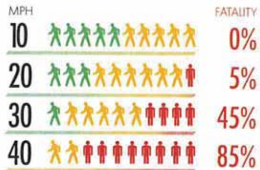
Figure 9. Speed and Crash Severity
